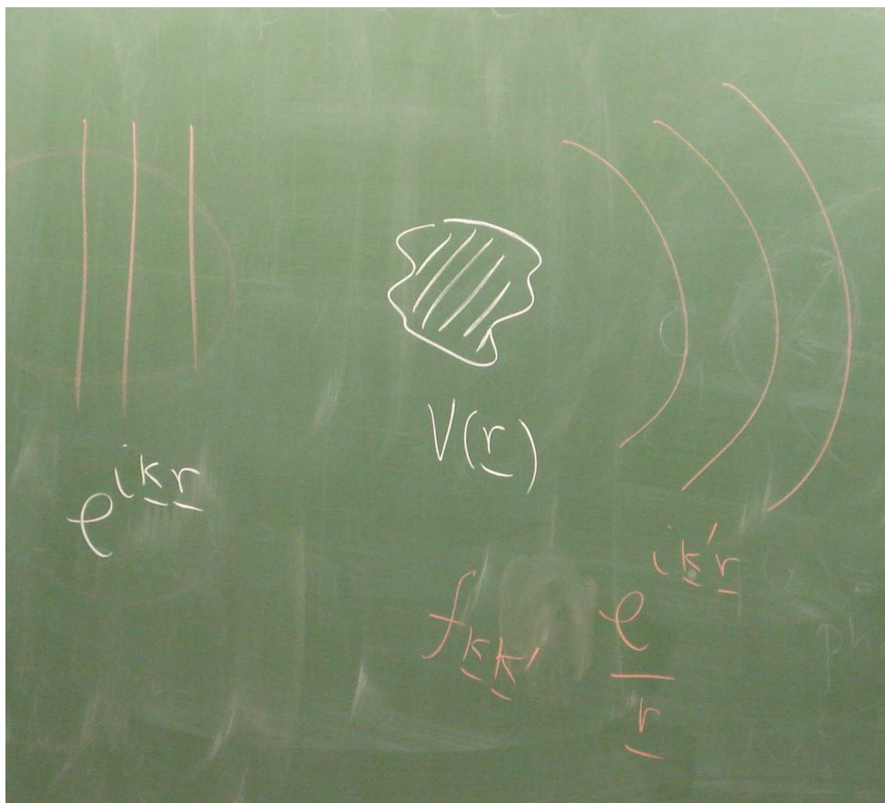
Figure 3. Scattering of a plane wave by a potential V(r) into spherical waves f_{\mathbf{k}}(\theta, \varphi) e^{i\mathbf{k}' \cdot \mathbf{r}}/r .
